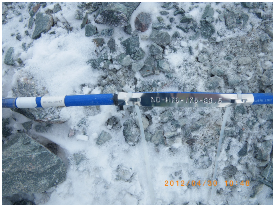
Photo 1: GTC ND-HTS-175-33.5 correctly labelled.
