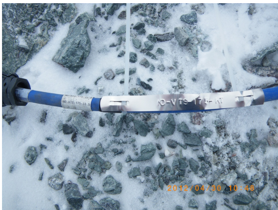
Photo 2: GTC ND-VTS-175-KT correctly labelled.
